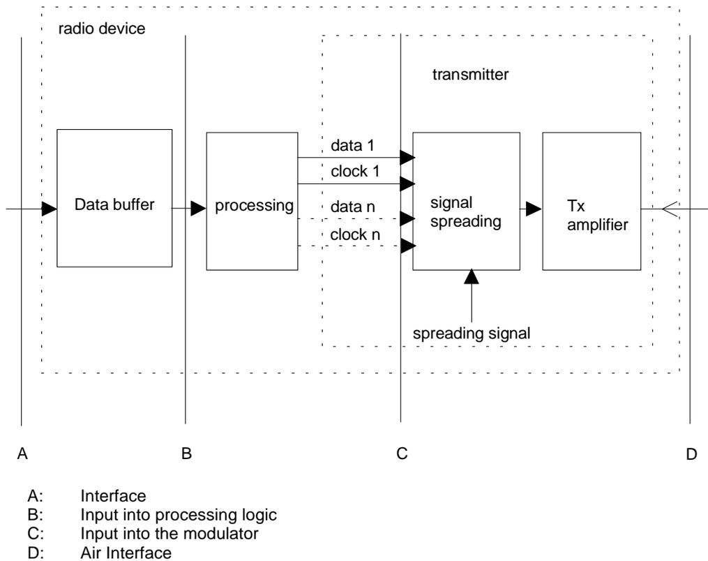
**Figure 1: Parameters related to the aggregate bit rate**
